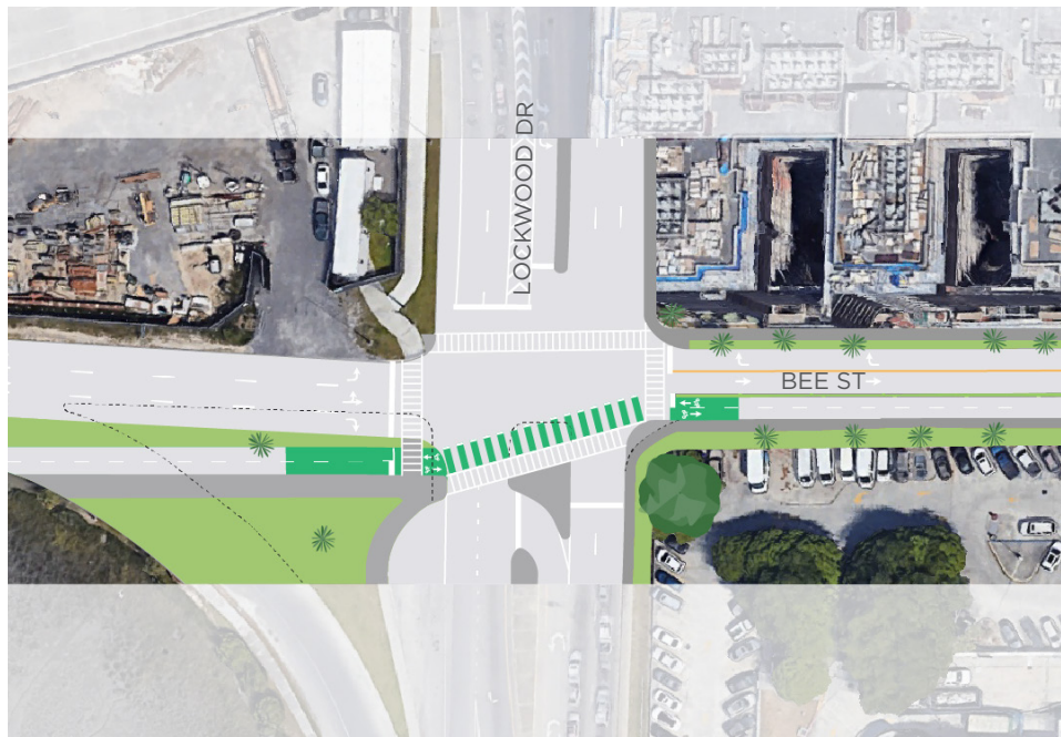
Alternative 3: Angled cycletrack crossing, right turn lane onto Lockwood Drive, angled pedestrian crosswalk
