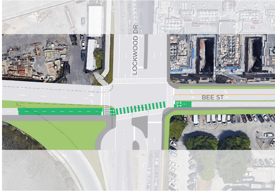
Alternative 2: Angled cycletrack crossing, slip lane onto Lockwood Drive, straight pedestrian crosswalk
